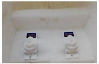
Make Z-bendings on the pushrods and insert them into the sleeves with Z-bendings from the outside.
