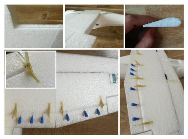
The inner and outer flaps are connected by a piece of wire and pushrod plastic tubes.
