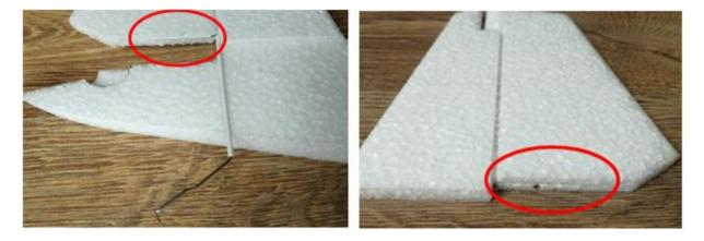
Prepare one more channel in the right-side fuselage part for the servo cables that go from the wing to the receiver, see picture.
