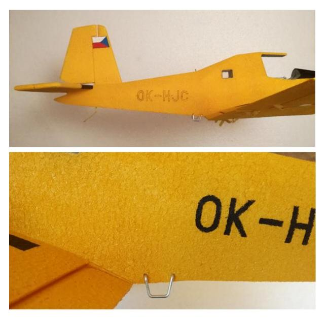
It is recommended to attach wire to the wing ends from below to protect them from contact with the ground.
