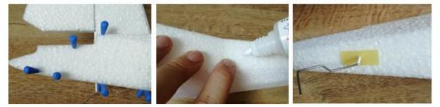
Insert the control horn in the elevator onto the pushrod Z-Bend and place the horizontal stabilizer on the fuselage according the center line.
