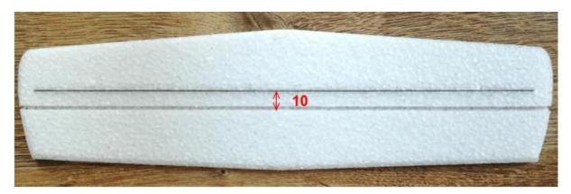
Place the horizontal stabilizer on one part of the fuselage (with the control horn in the elevator facing the inside of the fuselage) and mark the position where the control horn will move during elevator operation (with enough space around the control horn).
