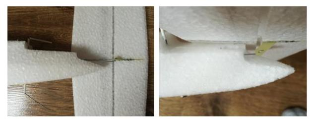
Glue the vertical stabilizer after the glue on the horizontal stabilizer is dry. First glue it to the fuselage and check that it follows the center line of the fuselage and is perpendicular to the horizontal stabilizer. Then glue the tail landing gear wire to the underside of the rudder with the installed plastic tube. Slide the longer control horn onto the pushrod Z-Bend and glue it also to the bottom side of the rudder. **Beware that no glue flows in the plastic tube!!**
