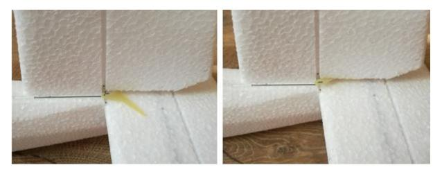
We recommend using the Emax CF 2812 motor, as no further modifications have to be made to the fuselage. The motor mount (supplied with the motor) is installed in reverse order, so it is shorter, see picture.
