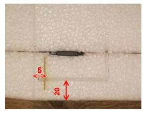
deep as the groove in the stiffener. It is recommended to apply some narrow tape to the plastic pipes on the corners of the landing gear (marked in the picture below) so that no CA glue can flow into the tubes, because the wire must remain freely movable in the pipes, otherwise the landing gear will tear from the wing during harder landings. This ensures a torsional suspension of the landing gear. The landing gear can be glued after painting the model.
