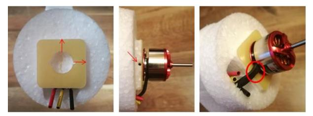
Connect the motor ideally with connectors to the ESC and check the correct direction of rotation. Hollow out a small opening for the cables in the engine cowling and attach it with a few drops CA to the fuselage. Paint the engine "shutters" silver and press them after painting the model in the cowling. The shaft of the motor should come out approximately in the center of the "shutters" with the correct side-thrust and down-thrust.
