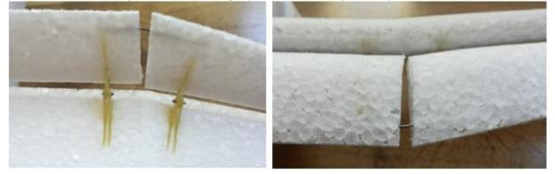
Pierce a piece of pushrod tube near to the trailing edges of the flaps to be connected (parallel to the trailing edge) so that they can be connected by a piece of bend wire. Glue the tubes from the outside carefully.
