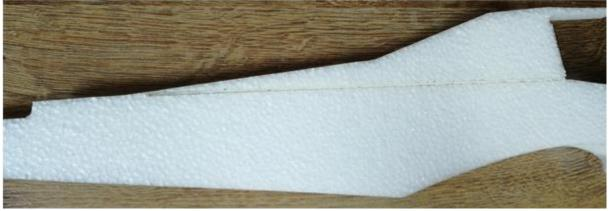
Now prepare the cavity for the receiver in both fuselage parts behind the cockpit. It is best to use a transformer soldering gun with a long wire. Leave a wall between the receiver cavity and the cockpit, it will be cut out after the fuselage is glued together and then put back in place.
