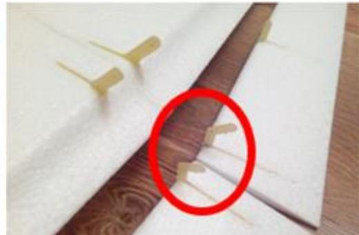
Before gluing all the hinge-levers into the wing and flaps, push a long piece of steel wire through all hinges of each flap in order to level the hinges and properly align the flaps with the wing. (Check for ongoing trailing edge and maintaining the shape of the airfoil). Glue all the hinge parts with thin CA.
