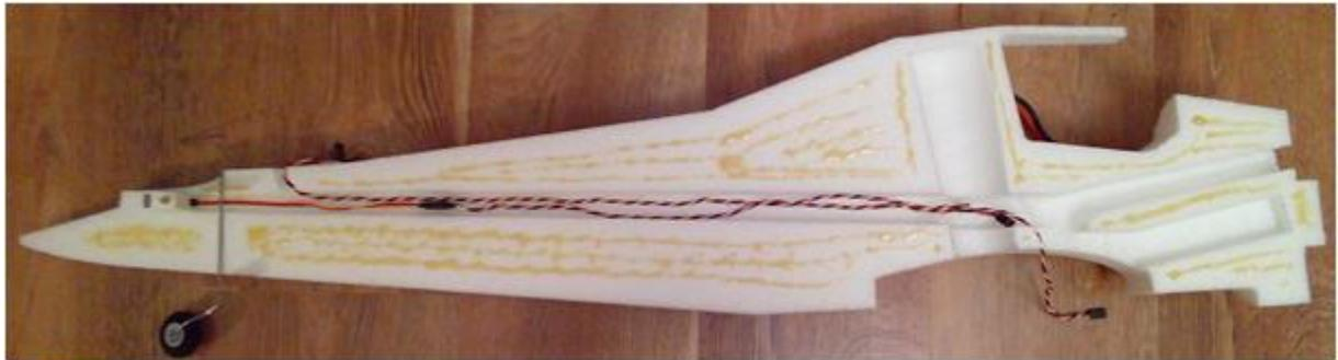
Glue together both parts of the horizontal tail surface and reinforce it with a 5x0.6 carbon stringer along the entire length from one side. Cut and glue the control lever into the elevator in the servo lever axis using CA (1 from 4 pcs - different shapes than those used as the flap hinges). Carefully glue the horizontal tail surface to the fuselage with PU + CA glue. Before applying CA, check the perpendicularity to the fuselage.
