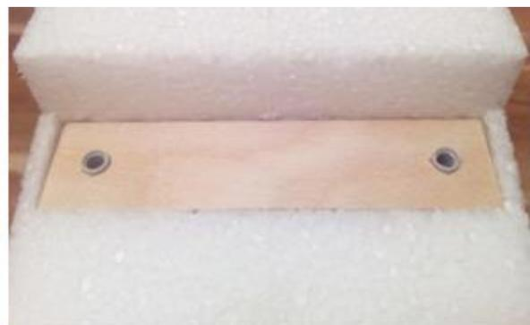
Roughen the engine bulkhead and glue it with the cable cutout to the upper side. The mounting holes for the engine are drilled asymmetrically for setting the downthrust and sidethrust of the engine, and it can therefore **only be glued with one position** - the engine shall be placed more in the top-right corner as viewed from front. Mount the engine and align it slightly to the right and downward (spacer  $\pm 4$  mm in the top-right corner as viewed from front).
