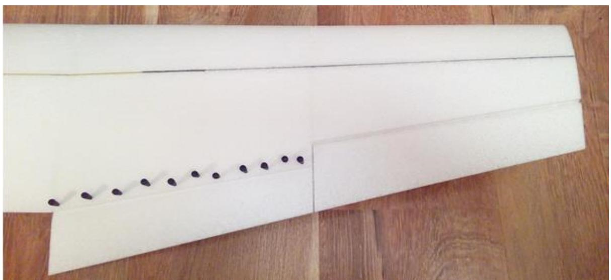
Cut slots at a right angle into the flaps at a distance of 120 mm for the 90° levers creating hinges (shorter inner flaps in the wing mid section - 130mm distance). Use the extended levers in the flaps (for flaps control) on the place, where the wing mid section is joined with the outboard wing section. Cut slots into the wing for the opposite parts of the hinges, which have to be glued together according the following image (push two pieces of wire through the parts, then glue them together) →
