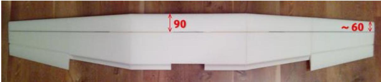
Cut the slot for the spars and stringers on the upper side of the wing in the same way. (Make the slot for the spars with a sharp knife and push them in - you can use a small hammer). Level the wing on a flat surface (table or floor), check the wing is straight and with the same dihedral on both wing tips, then glue the spars and stringers into the wing with thin CA glue.
