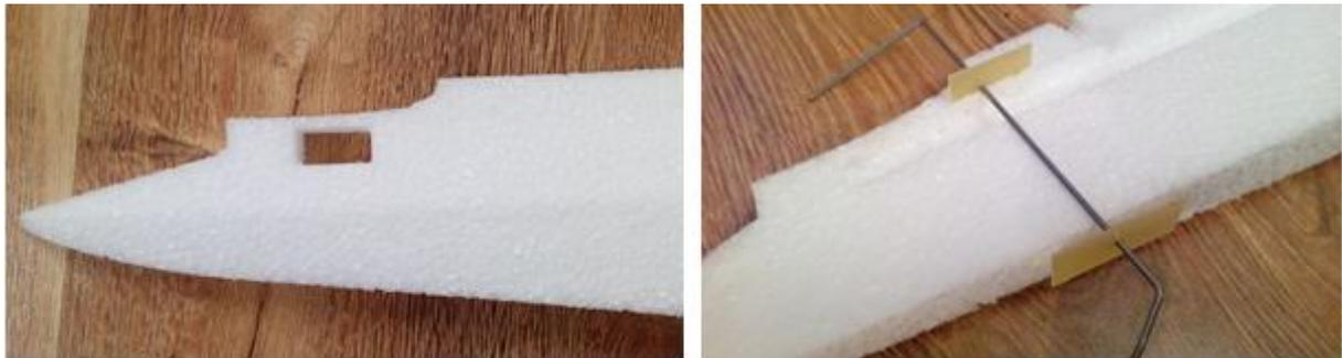
Scoop out enough space for the Electronic Speed Controller in the front bottom part of the fuselage. Lead the groove for the power cables above the wing and forward to the engine bulkhead. Do the same for the battery.
