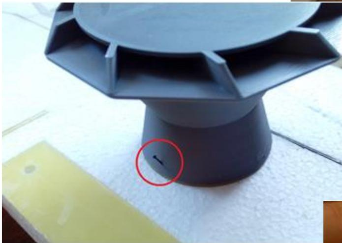
Included in the spreader set is the hopper cover. After painting, bend 2 pieces of wire to form a "U" shape, push them thru the eyelets, insert and glue them into the EPP.
