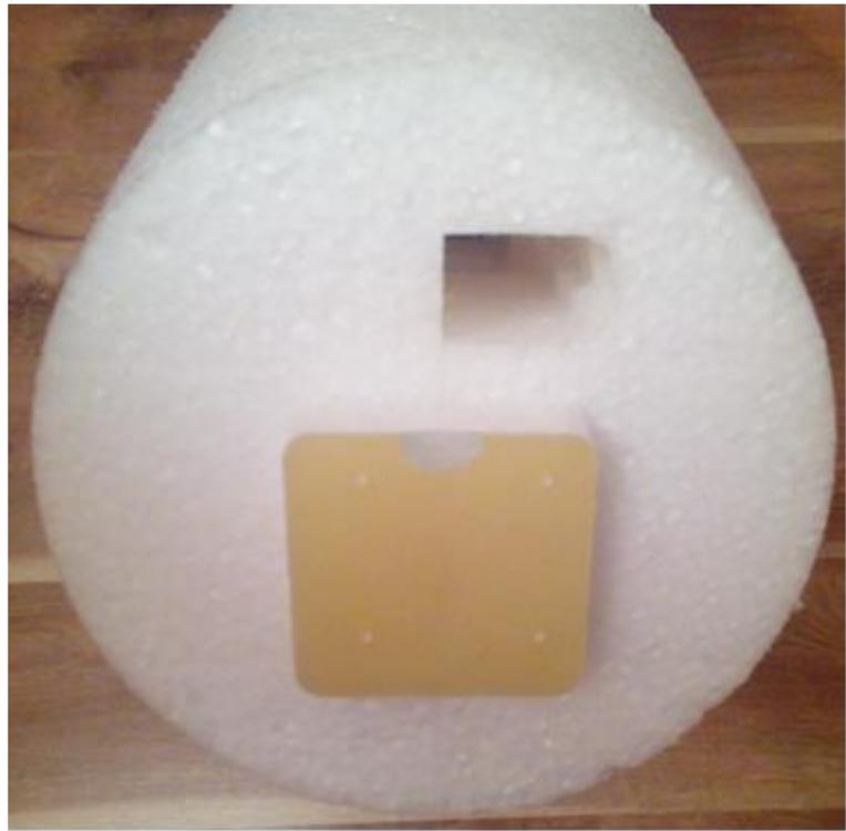
Carefully glue the remaining fiberglass plate to the fuselage as a reinforcement of the tail landing gear, avoiding gluing the wire itself. Secure the wheel with the stop collar.
