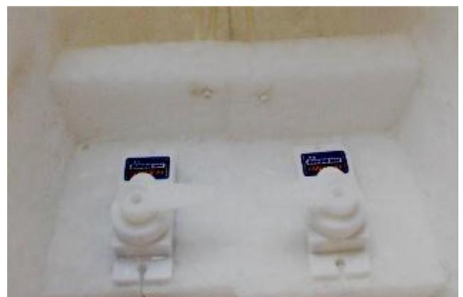
**Note:** Both pushrod sleeves from the elevator are leading to the R.H. servo (in the direction of flight).
