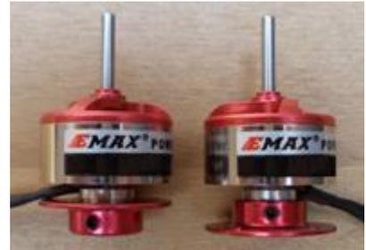
After soldering of the wires between the motors and the ESCs test the sense of rotation, the motors have to be counter-rotating, the left motor has to turn clock-wise and the right one counter-clock-wise in the direction of flight.
