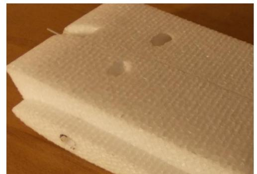
Glue a carbon rod 1 mm dia. between the parts „4“ and „5“ – wing tip tanks. Extend the wing profile cutout in the part „4“ till the trailing edge of the wing. Glue them to the end of the wings.
